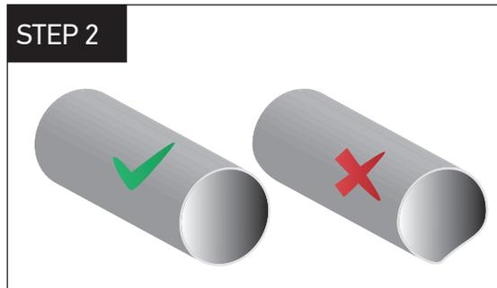
Primex recommends using a diffuser collar to counter vent warping and improve retention in the duct.
